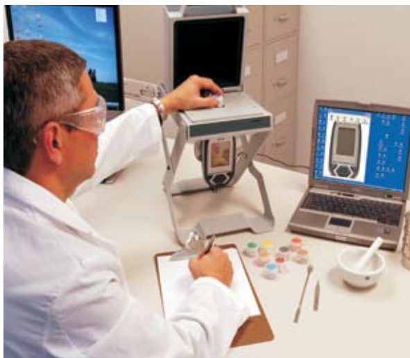
Test stand converts instrument to provide screening of prepared samples, dramatically increasing throughput.
