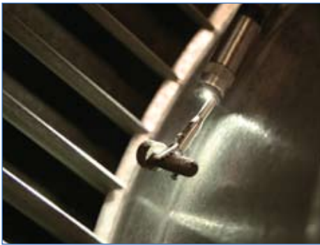
Bolt retrieval using 3 mm Alligator working tool
